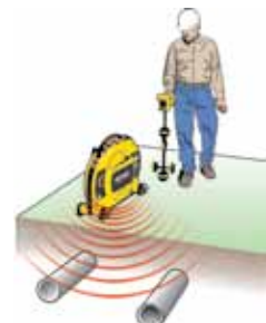
Induce a signal to locate utilities.
